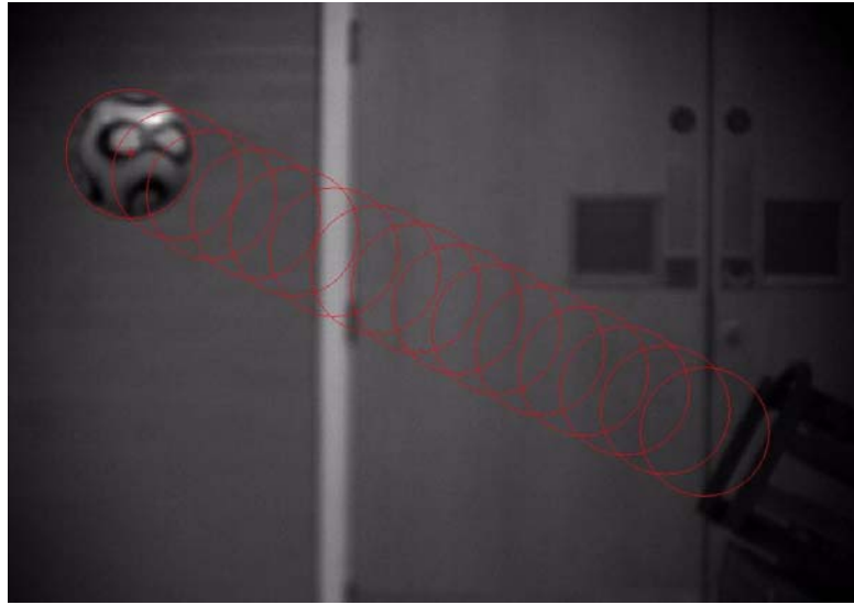
Figure 4. Data from camera 1 for a launch with backspin. Each circle's centre denotes the ball's centre of mass in 0.005 s intervals. The ball was launched with the speed of 15.8 \text{ m s}^{-1} at an angle of 27.2^\circ above the horizontal. Its 84.9 \text{ rad s}^{-1} (811 rpm) angular speed meant that Sp \simeq 0.59 . (This figure is in colour only in the electronic version)
